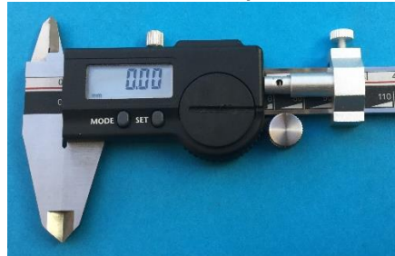
A40 mounted on a caliper with roller
