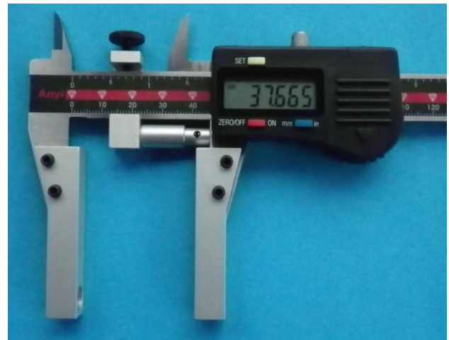
Caliper no. 110-051 mounted with FMS insert holders type 10A and pressure device 40A for internal measurement ready for FMS inserts.
