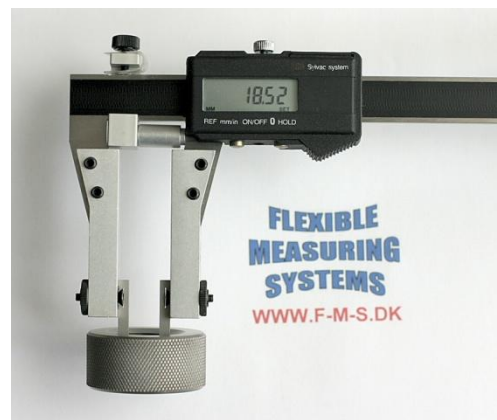
Measuring internal thread pitch diameter
