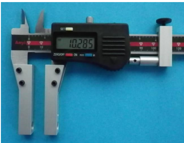
Caliper no. 110-151 with a resolution of 0.005mm/0.0002" and an accuracy better than standard with FMS insert holders 10A and pressure device no. 40A N.B. This caliper has a preset function.
