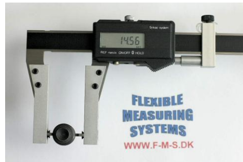
Measuring external thread pitch diameter
