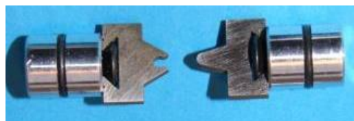
FMS external thread inserts. The inserts shown are no. 21B and cover the range of 2-4 mm / 13-6 TPI
