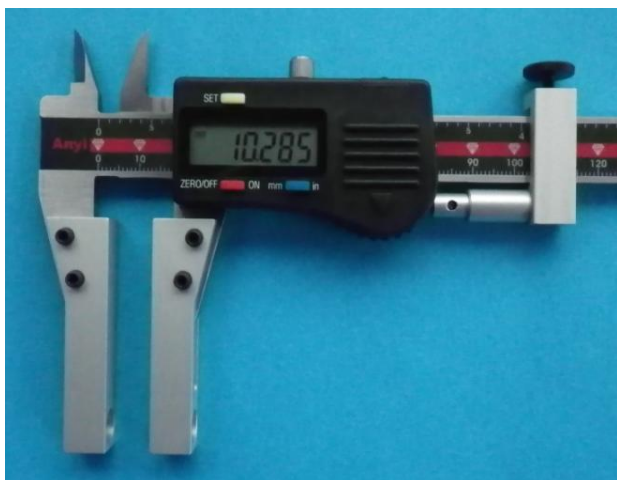
A caliper with a resolution of 0.005mm/0.0002" and an accuracy better than standard with FMS insert holders 10A and pressure device no. 40A
