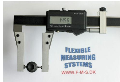
Measuring external thread pitch diameter
