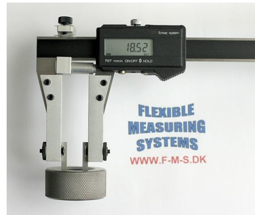
Measuring internal thread pitch diameter
